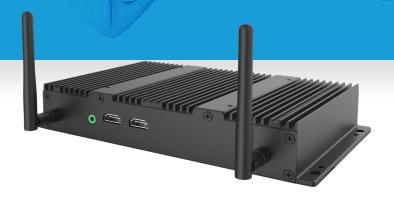
The Element KPC6 is an ultra-thin, embedded Box PC, crafted from diecasting aluminum, that has a fanless and ventless design. It can be mounted to a wall or placed behind a monitor, via a 100mm x 100mm VESA mount, to deliver high-graphic performance while using minimal power. The unit also offers dual video support via HDMI.
