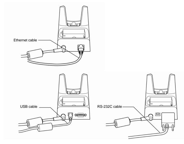
**4.** CU-1211: Connect the other end of the Ethernet cable to the Ethernet hub.
