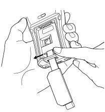
4 Insert a new hand belt (loop first) into the same slot.
