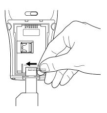
Insert the shaft pin through the loop.
