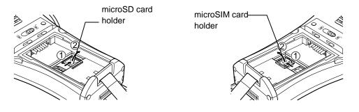
3. Insert the microSD or microSIM card into the card holder slot.
