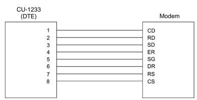
Cable connection between CU-1233 and modem
