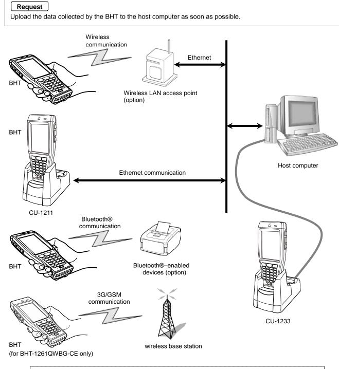
A wireless local area network between the BHT and wireless LAN access point is required to communicate via the wireless LAN.
