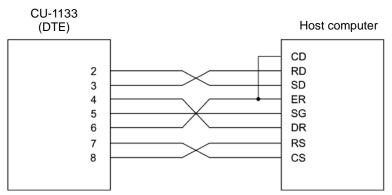
Cable connection between CU-1233 and host computer
