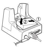
3. Remove the battery from the CU.
